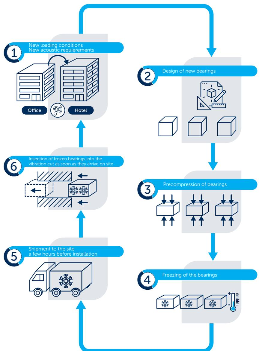
Figure 6 - Frozen Bearing Technology Process: Main Steps
