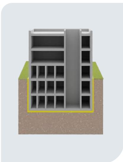
Figure 4.1 - Decoupling the entire building from the soil
