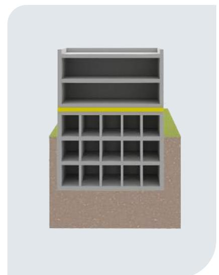
Figure 4.3 - Decoupling at floor level
