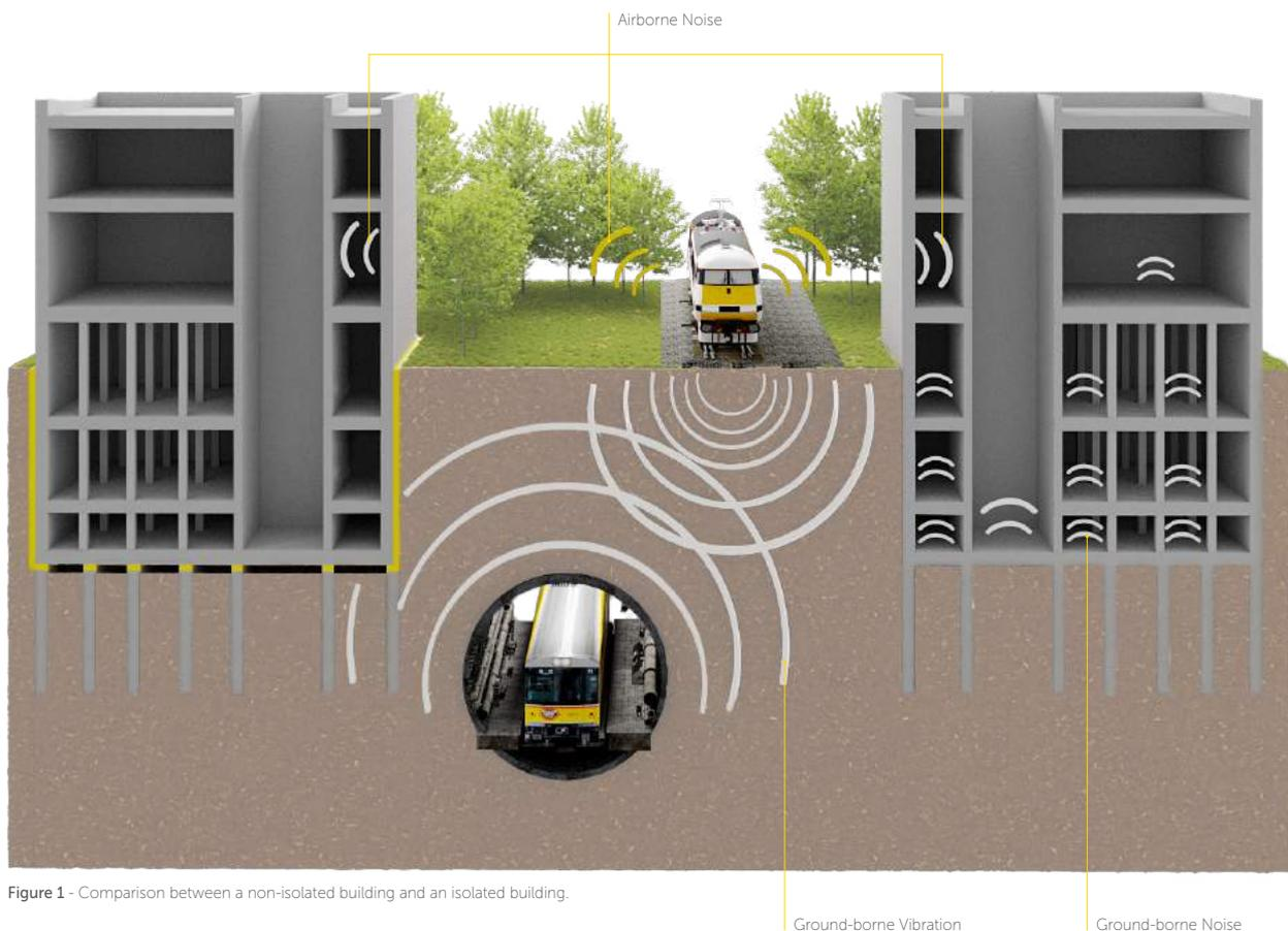
Figure 1 - Comparison between a non-isolated building and an isolated building.
