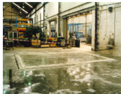
CDM-ISO-Machine Float with inertia base sunk into the ground
