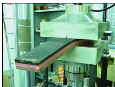
Dynamic stiffness test on the triple strip
