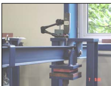
Creep test on the triple strip
